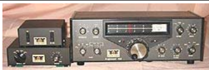
The Argonaut 515, Model 206A Crystal Calibrator (frequency marker) and Model 208A three-position crystal and notch filter.
