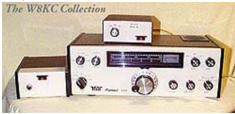
Front view of the Ten-Tec Argonaut 509. The physical appearance of the 505 and 509 models is almost identical. Matching accessories: On top of the radio is the Model 208 CW filter. At the left is the Model 210 power supply (1 A regulated). [Courtesy of the Virtual Ten*Tec Museum .]
