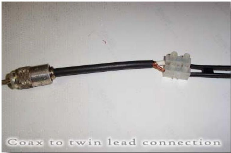
possible to use the antenna on 160 meters but you will need to connect the twin lead together at the point where it connects to the coax. On 160, the antenna performs like a Marconi. Those who have used the antenna on 160 say the "GI Mystery" antenna is a quieter receiving aerial compared to other 160-meter antennas.
